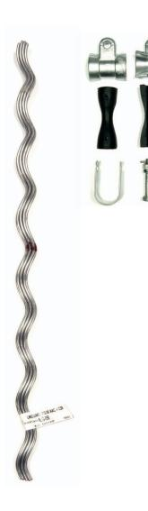
The Preformed Armor-Grip Suspension unit is intended for use on all material types and conductor constructions. Designed to reduce the static and dynamic stresses at the support point so that the conductor is protected against the effects of conductor motion. It also protects the conductor in the support area against impulse and power flash-over arching.
